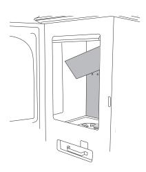
4. After that take out the angle-brick Now it's easy to remove the rest of the bricks.
