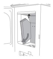
2. Then remove the big side-brick by first lift the roof brick that lock the big-side brick
