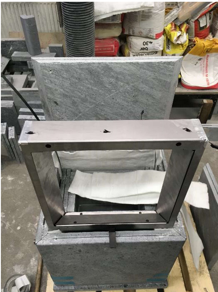
Use silicone dots for 30 mm stones
