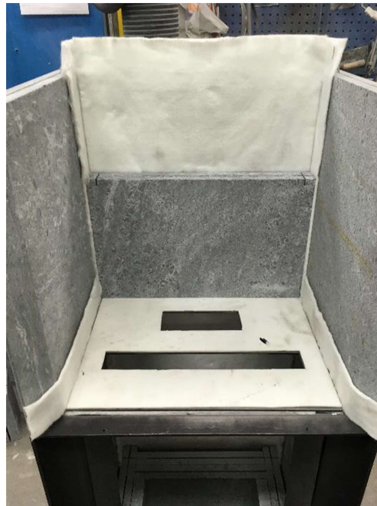
Install back stone (stone order will be changed)
