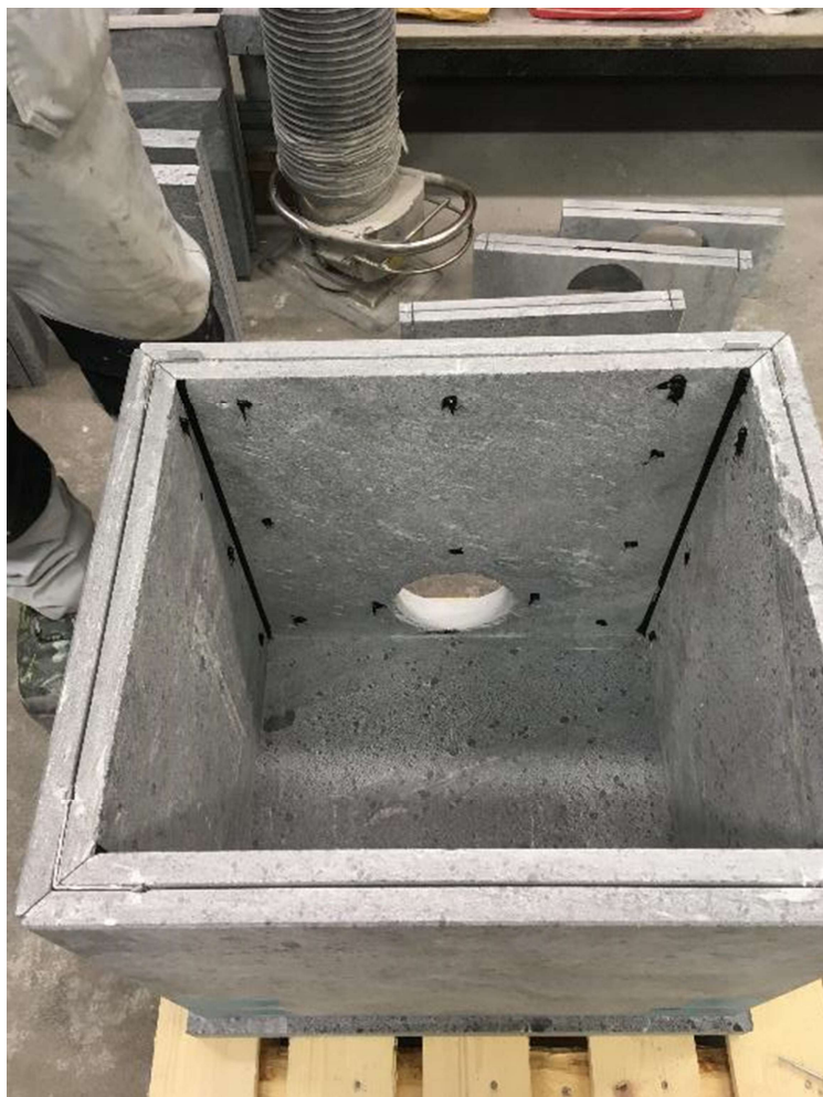
Put silicone dots for wool
