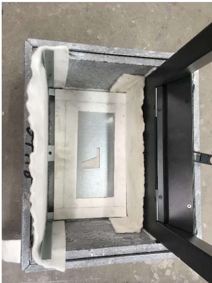
Tigh with wools and put ceramic paper in bottom
