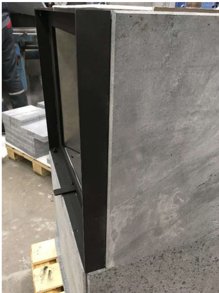
Tighten door so, that there approx.1 mm gab
