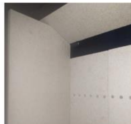
6. Place left side brick. Make shure that inner baffle is placed in its rightht position on top of the side brics.
